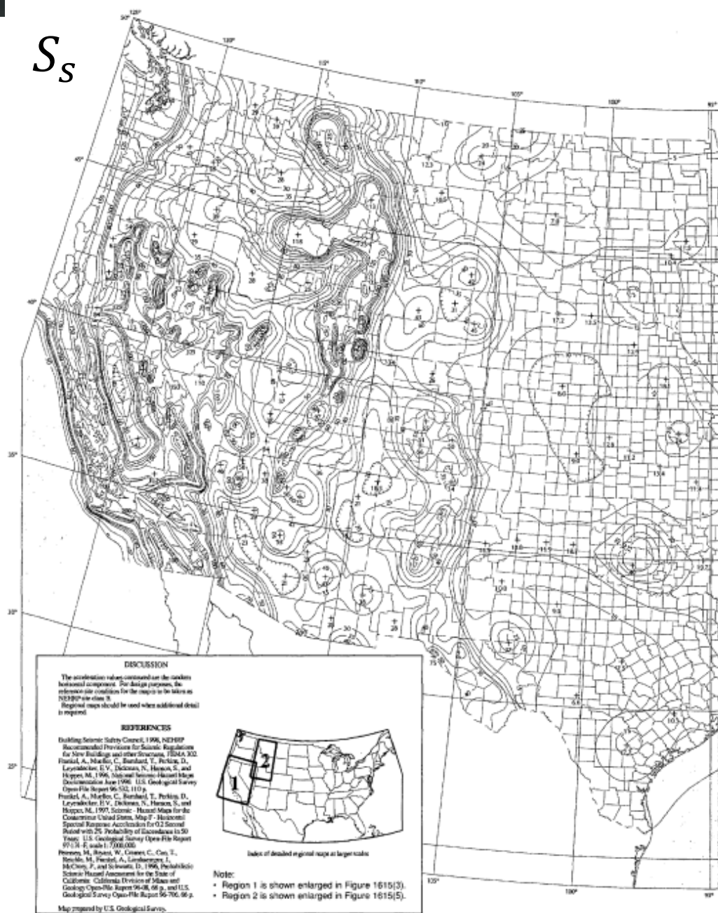
FIGURE 1615(1) MAXIMUM CONSIDERED EARTHQUAKE GROUND MOTION FOR THE CONTERMINOUS UNITED STATES OF 0.2 SEC SPECTRAL RESPONSE ACCELERATION (5 PERCENT OF CRITICAL DAMPING), SITE CLASS B
