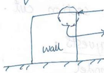
In actual tests, we have a beam on top of wall and we push that beam. In model also, add rigid plate to avoid local deformation.
