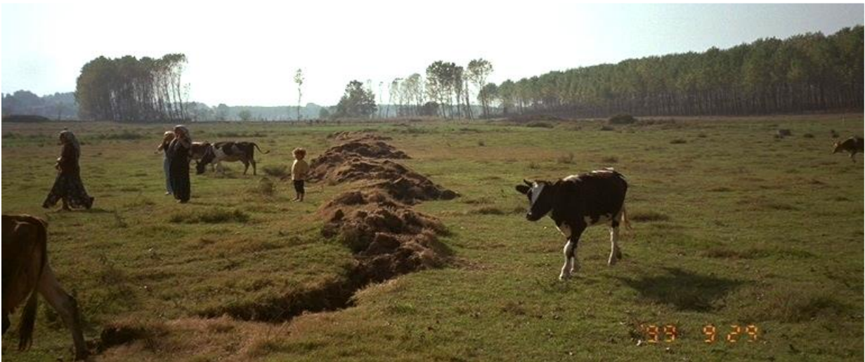
Ground Failure by Lateral Fault Movement
