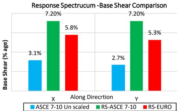
Figure 4. RS-Base Shear comparison (DBE-Level)
