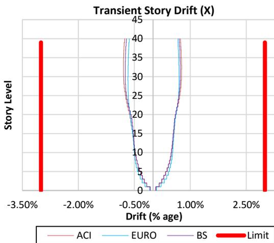
Figure 15. Transient Story Drift (X-MCE level)
