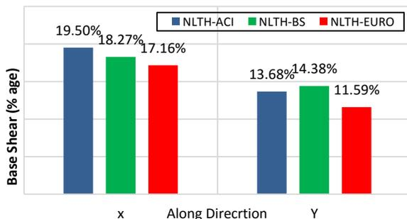
Figure 11. Nonlinear (NL) base shear expressed as a percentage of total seismic weight
