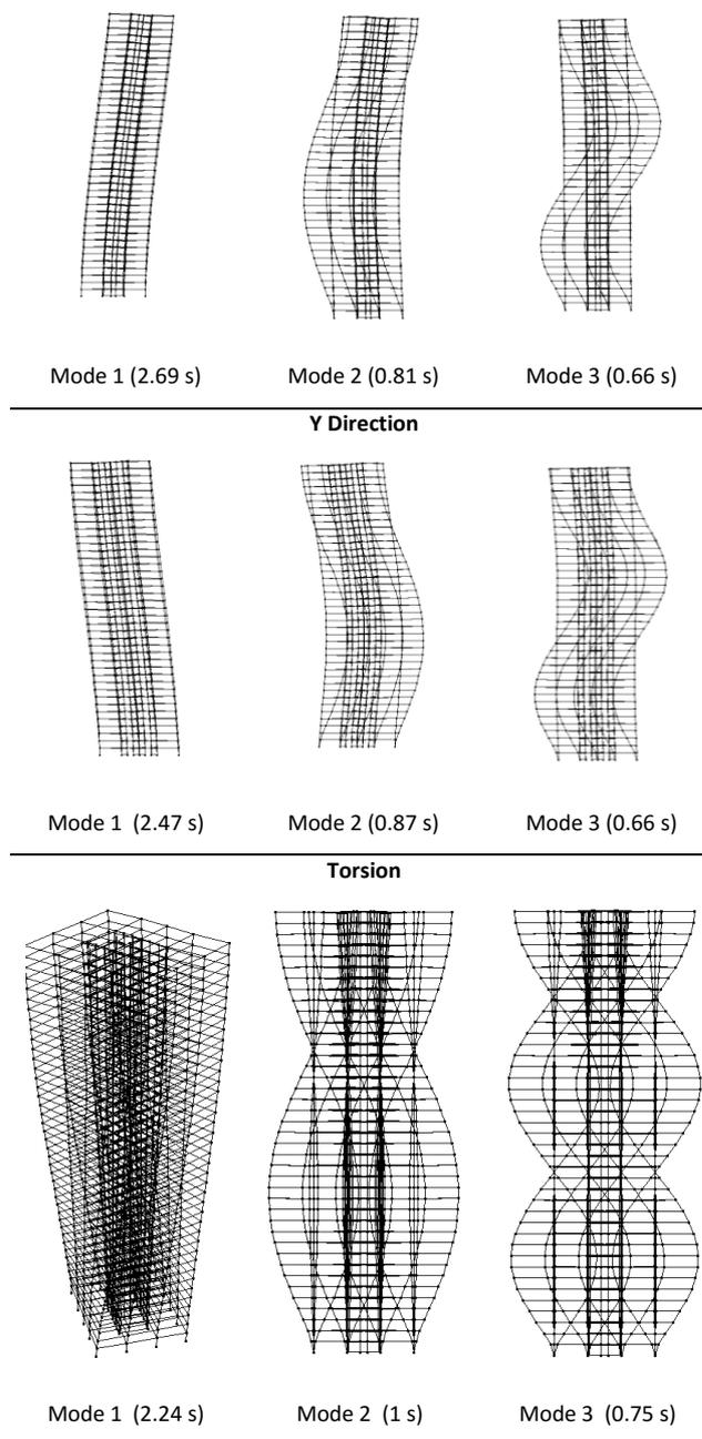
Figure 3. The vibration mode shapes
