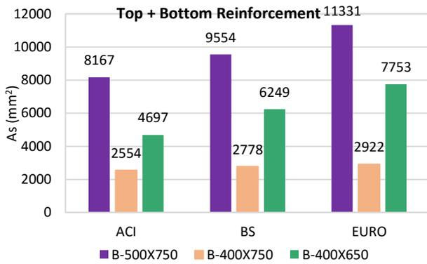
Figure 10. Beams reinforcement
