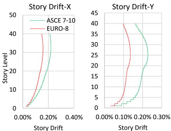
Figure 6. Story drift (X, Y Directions ) DBE Level)
