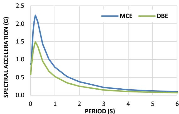
Figure 2. The DBE- & MCE-level response spectra used in this study
