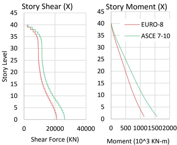
Figure 5. Story shear and moment comparison (X-DBE Level)
