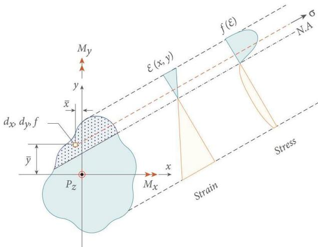
**Fig. 2** Strain and stress on a cross-section made up of a single shape and material, subjected to bending about an arbitrary axis
