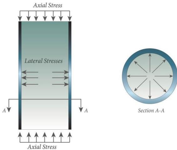
**Fig. 6** The development of lateral stresses in a concrete filled steel tube
