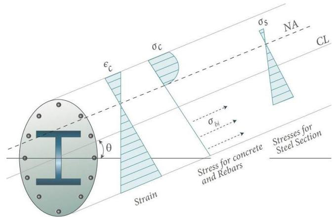
**Fig. 4** The stress resultants for a general cross-section made from several materials can be computed for a particular neutral axis angle direction and depth by first using assuming a strain profile, then computing stresses in each material at various location and then summing them
