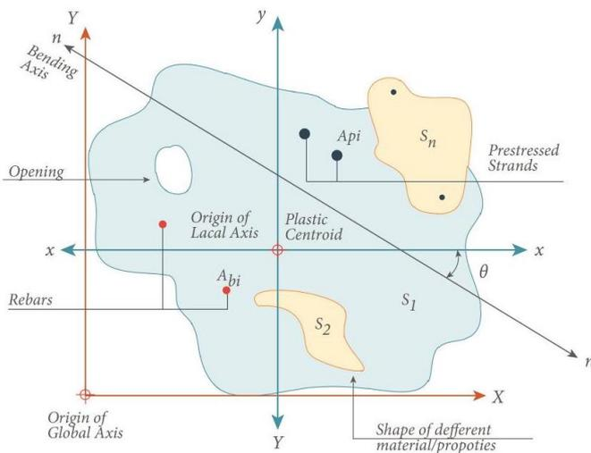
**Fig. 5** A generalized representation of cross-section having several shapes and materials
