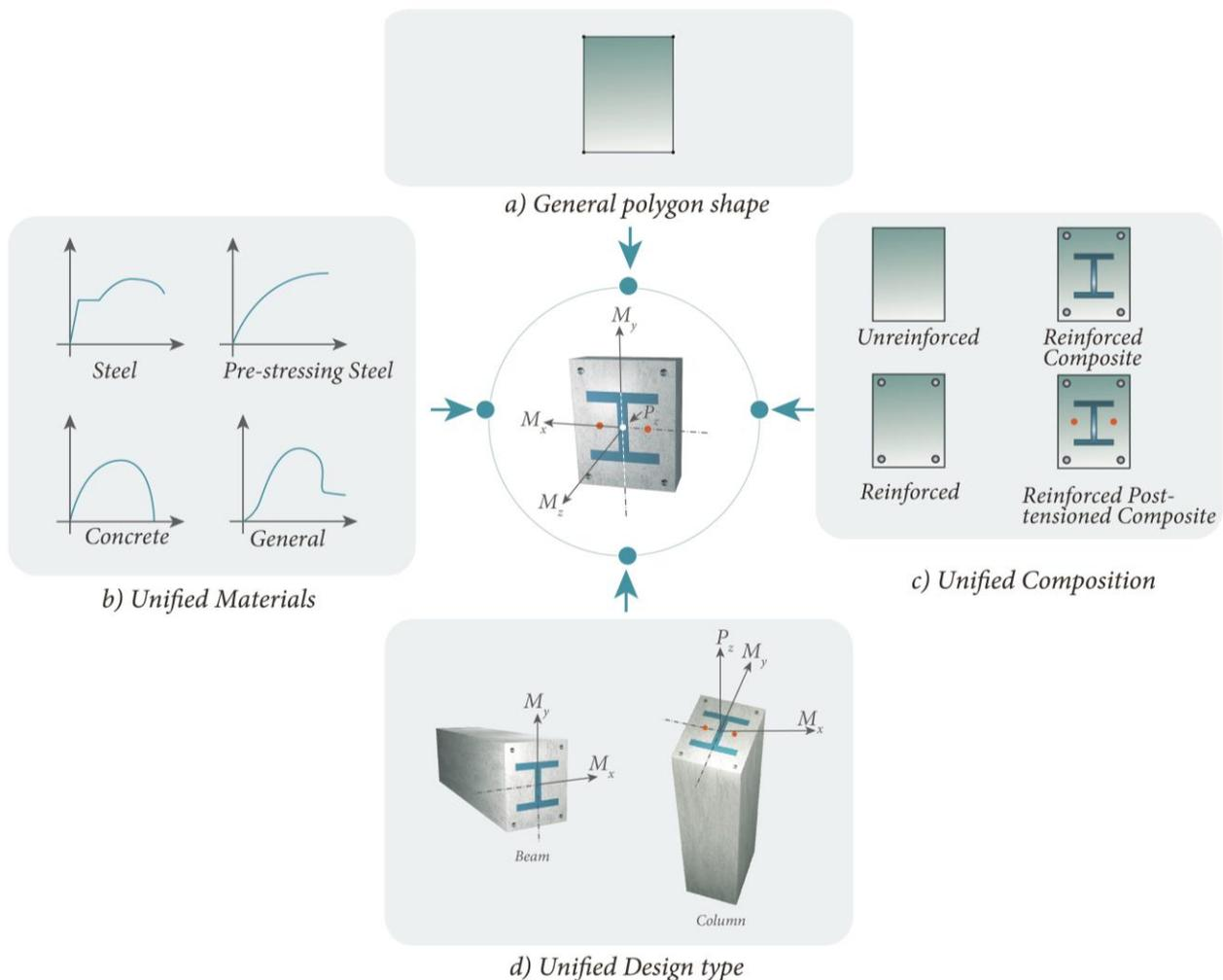
**Fig. 1** A general partially pre-stressed, composite beam-column cross-section, subjected to bending about arbitrary axis
