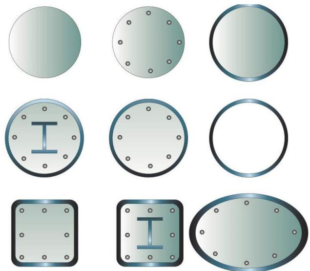
**Fig. 7** Various forms of concrete-filled steel tubes
