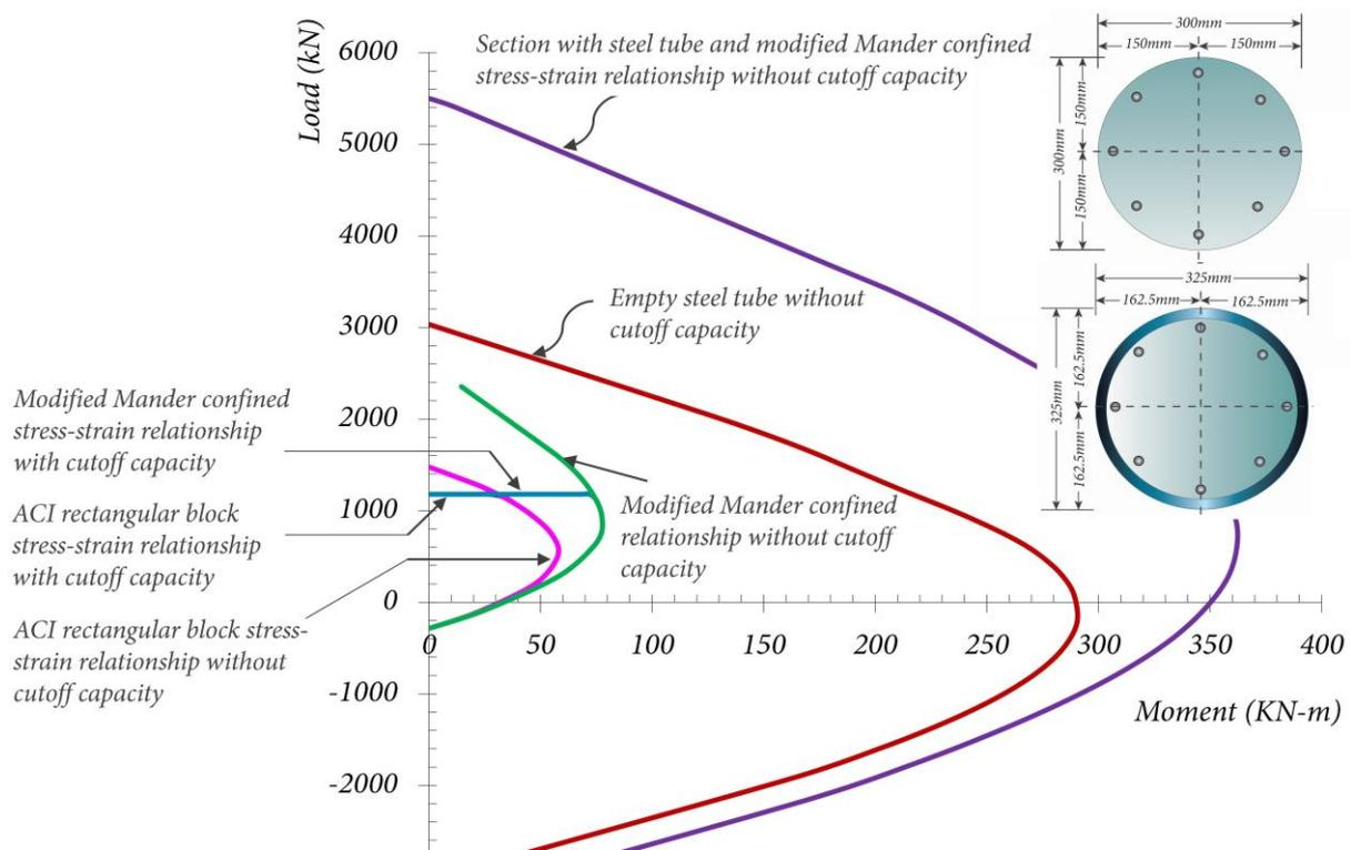
**Fig. 8** The effect of stress-strain relationship and confinement of concrete on the capacity of concrete filled tubes
