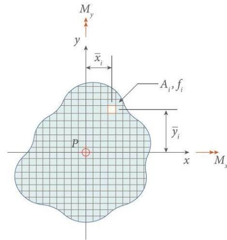
**Fig. 3** Stress resultants for a 2-D stress field using stress fibers
